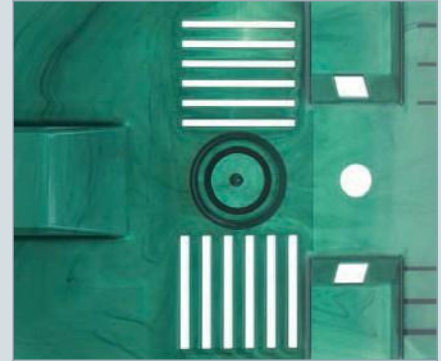
Colored streaks caused by the use of a screw with an unsuitable geometry
