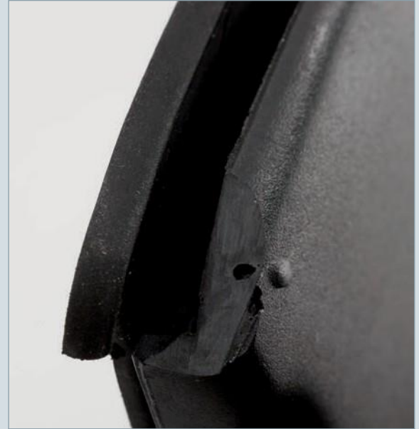
Air entrapment caused by an unfavorable molded part design
