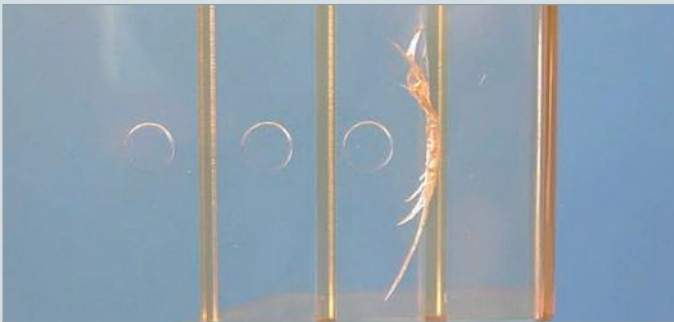
Rib without draft, asymmetrical arrangement of the ejectors
