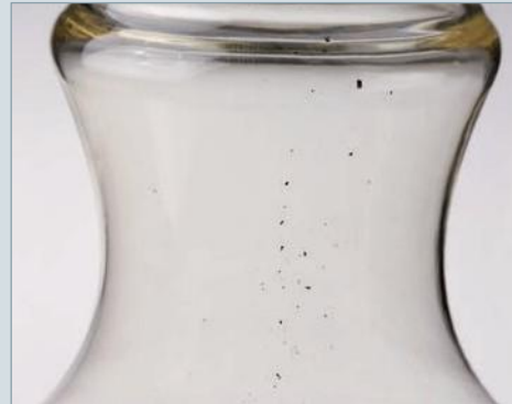
Impurities in a bottle due to dead spots in the plasticizing unit
