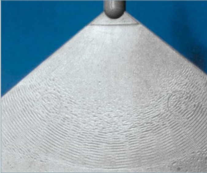
Record grooves effect because the melt temperature and the injection speed are too low
