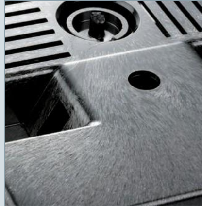
Moisture streaks in Ultrason®
