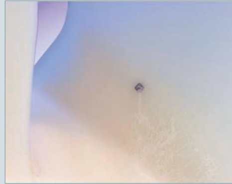
Black specks caused by foreign granules
