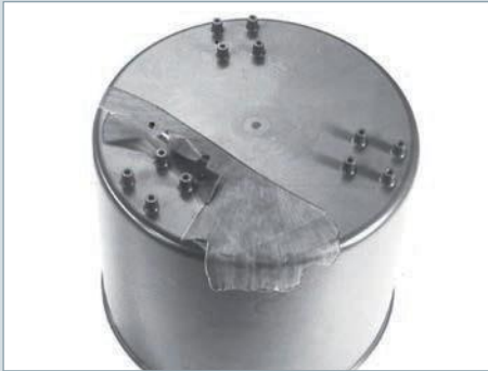
Delamination caused by an injection speed that is too high (mineral-filled Ultramid®)
