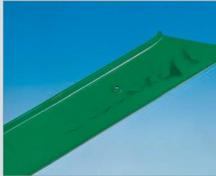
Colored streaks due to impurities in the hot runner
