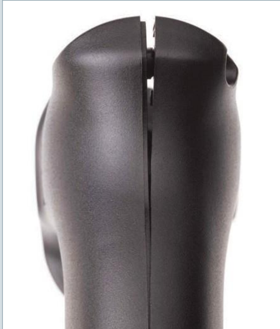
Warpage of a power drill housing made of glassfiber-reinforced Ultramic®
