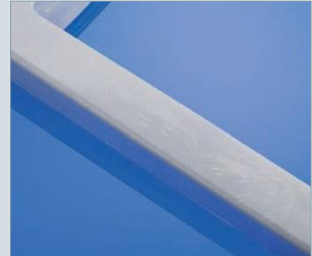
Streaks caused by thermal factors
