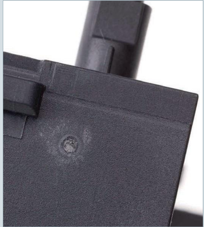
Dull spots in the area of the gate caused by high shear
