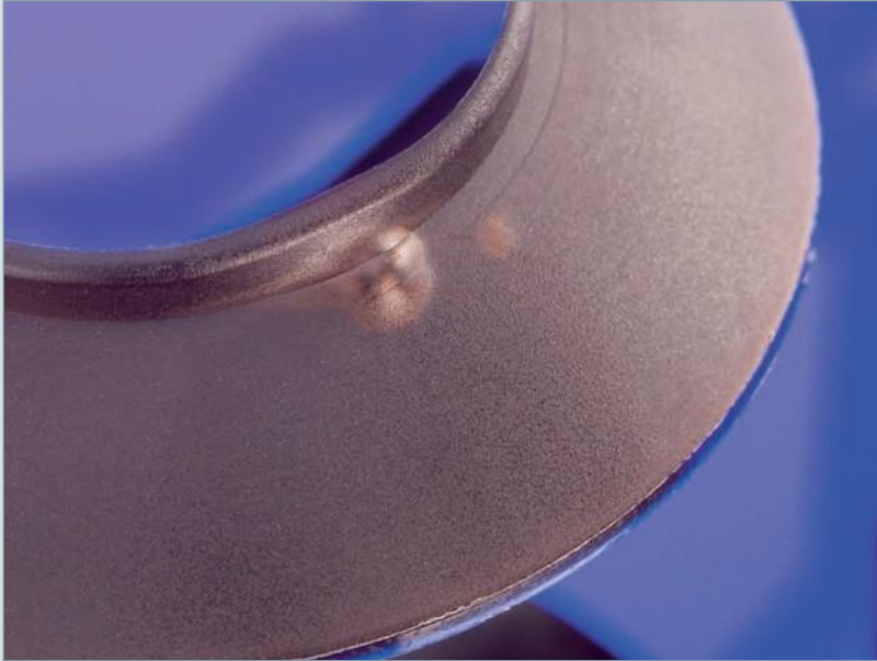
Air entrapment caused by entrapped air during the metering (unreinforced Ultramid®)
