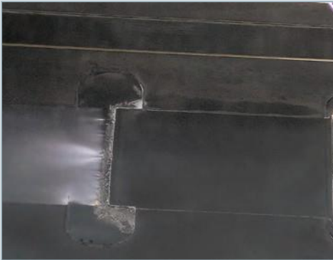
Plate-out/mold deposit at the dependent flow of path due to venting
