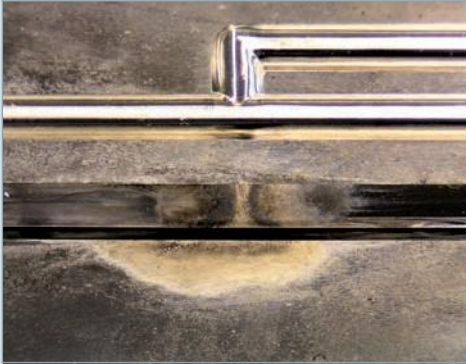
Plate-out/mold deposit in the area of a weld line due to a lack of venting
