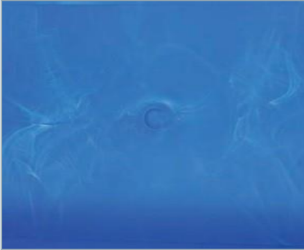
Colored streaks caused by the use of an unsuitable masterbatch
