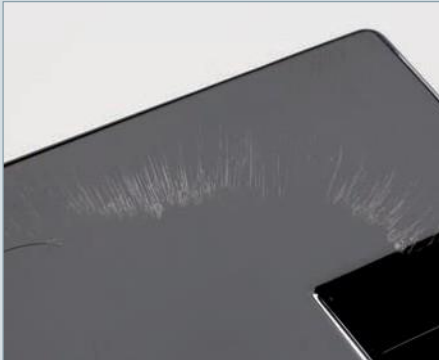
Burning streaks due to thermal degradation
