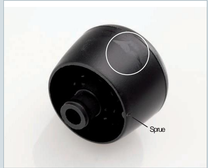
Cold slug in a molded part made of glassfiber-reinforced Ultramid®
