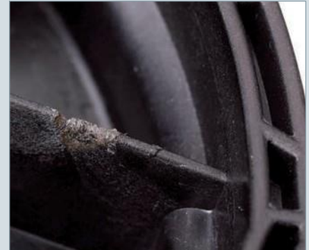
Diesel effect in a rib due to a lack of venting
