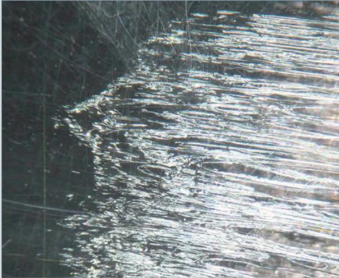
Streaks in Ultrason® caused by cold slug
