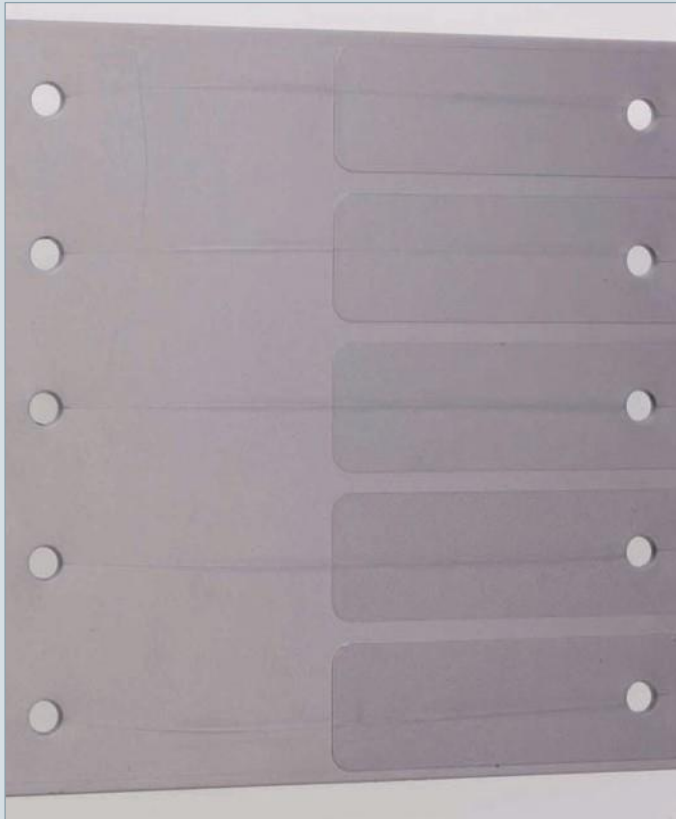
Weld lines after holes
