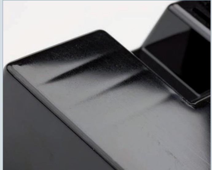
Sink marks caused by ribs
